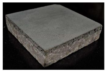
"HARDONATE METALTOP is graded, processed, nonoxidizing, non-rusting, inert metallic aggregate based floor hardener compatible with ordinary Portland cement."
